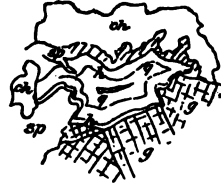
FIGURE 32.—Ore from the Moro mine, showing certain features of the paragenesis of the minerals. sp , Sphalerite; ch , chalcopyrite; g , galena; q , quartz; h , hematite.
